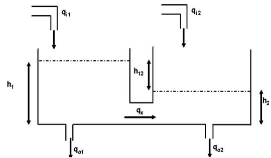
Figure 7: Coupled tanks model showing two tanks of water with heights  $h_1$ ,  $h_2$  and there difference  $h_{12}$ . Two inflow taps  $q_{i1}$ ,  $q_{i2}$  and two outflow plugs  $q_{o1}$ ,  $q_{o2}$  determine the flow in and out of the tanks and the cross-flow  $q_x$  describes the flow between them.
