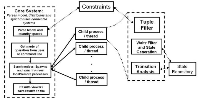
Figure 3: The JMorven Parallel Architecture.
